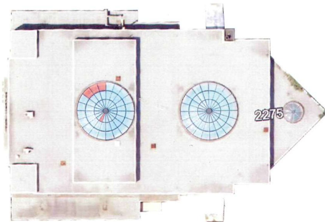
Figure 4: Damaged dome panels in need of replacement (highlighted in red)
