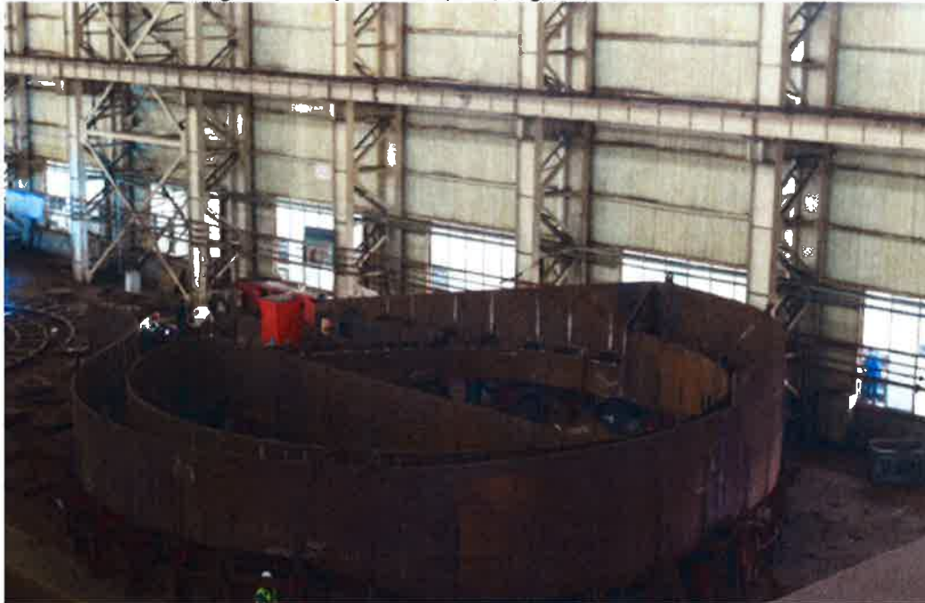
Photo 4 – Lower counterweight welding in progress
