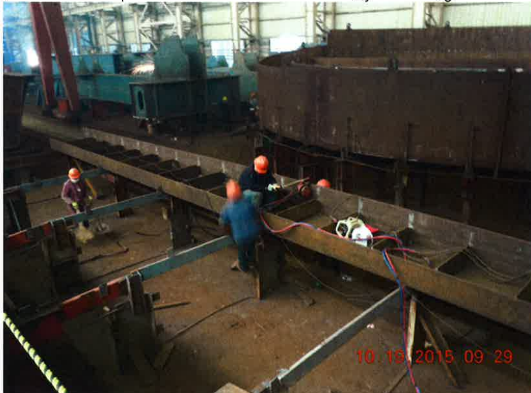
Photo 2 – Orthotropic steel deck end floor beam assembly and welding
