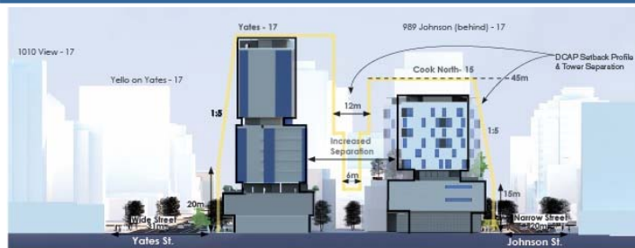
N-S BUILDING SECTION - POSSIBLE SETBACKS AND BUILDING HEIGHTS
