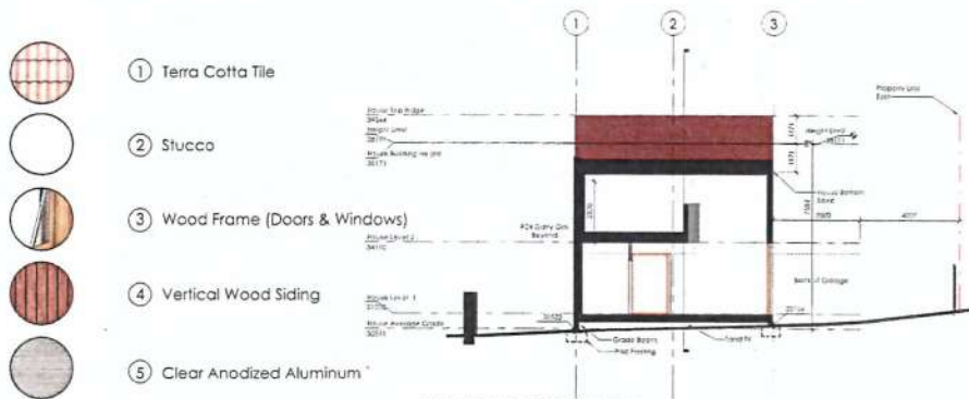
New House Cross Section South
