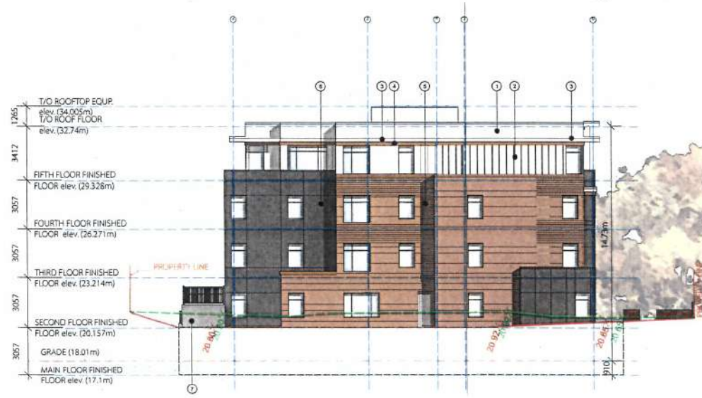
North Elevation SCALE 1/8" = 1'-0"
