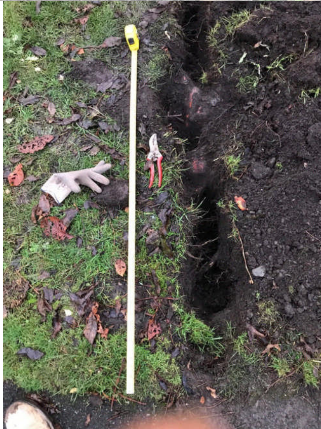
Photos #5 and 6: 15cm and 14cm roots were observed 5cm below the surface of the turf.
