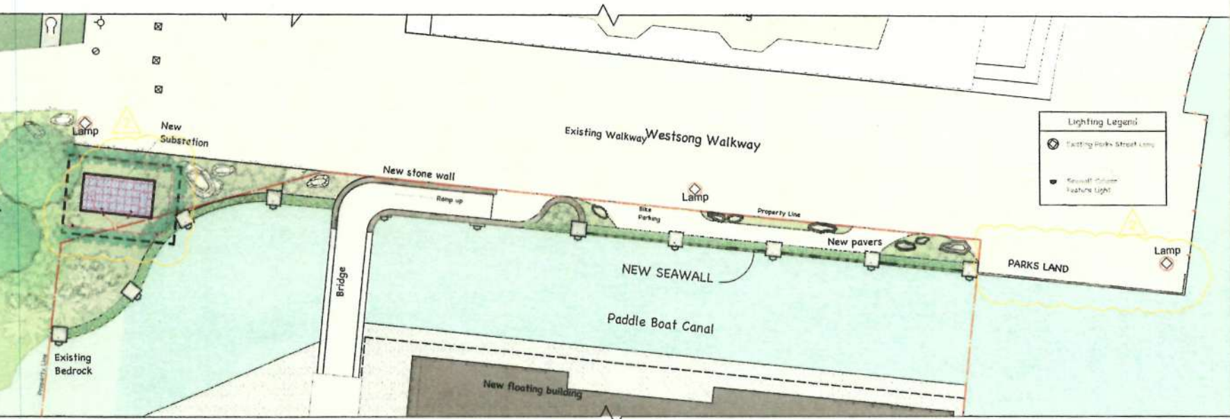
1 Proposed Seawall Plan (west side) Scale: 1:200
