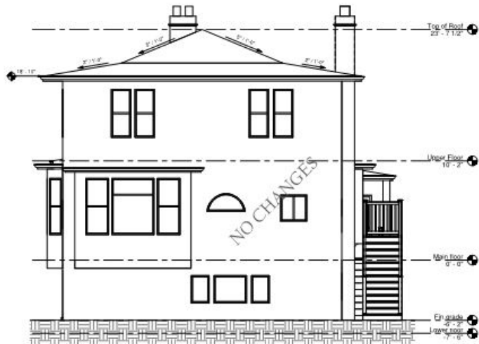
Existing Front Elevation 1/4" = 1'-0"
