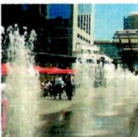
F2 BUBBLERS W/ NOZZLES FLYING IN GRADE
