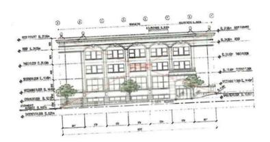
EAST ELEVATION CONTEMPLATED ALTERATIONS TO WINDOW OPENINGS
