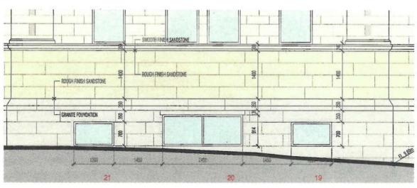
EXISTING NORTH ELEVATION - OPENINGS 19, 20 & 21 SCALE 1:50
