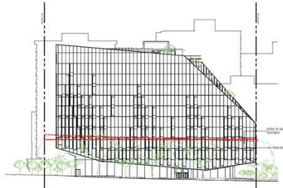
Elevations showing the extent of anti-collision treatment
