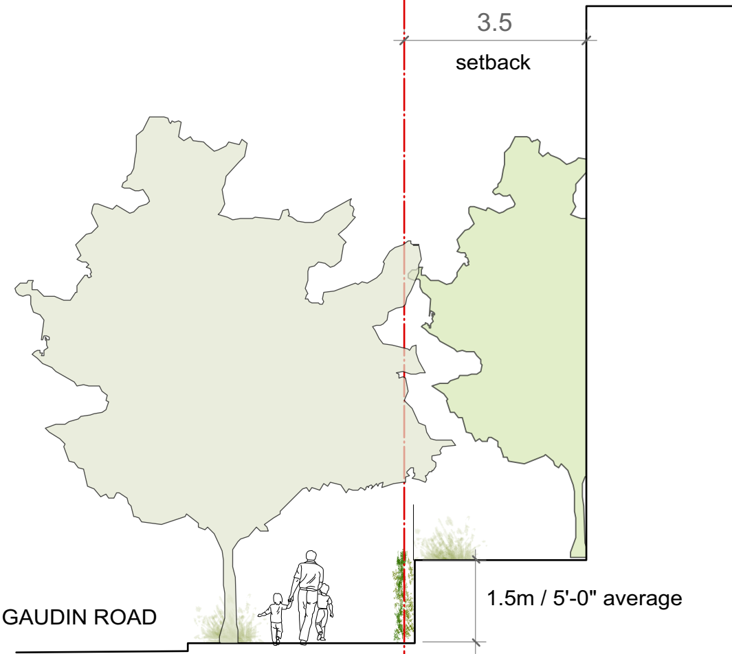
BUILDING PROFILE AT GAUDIN ROAD SCALE: 1:100
