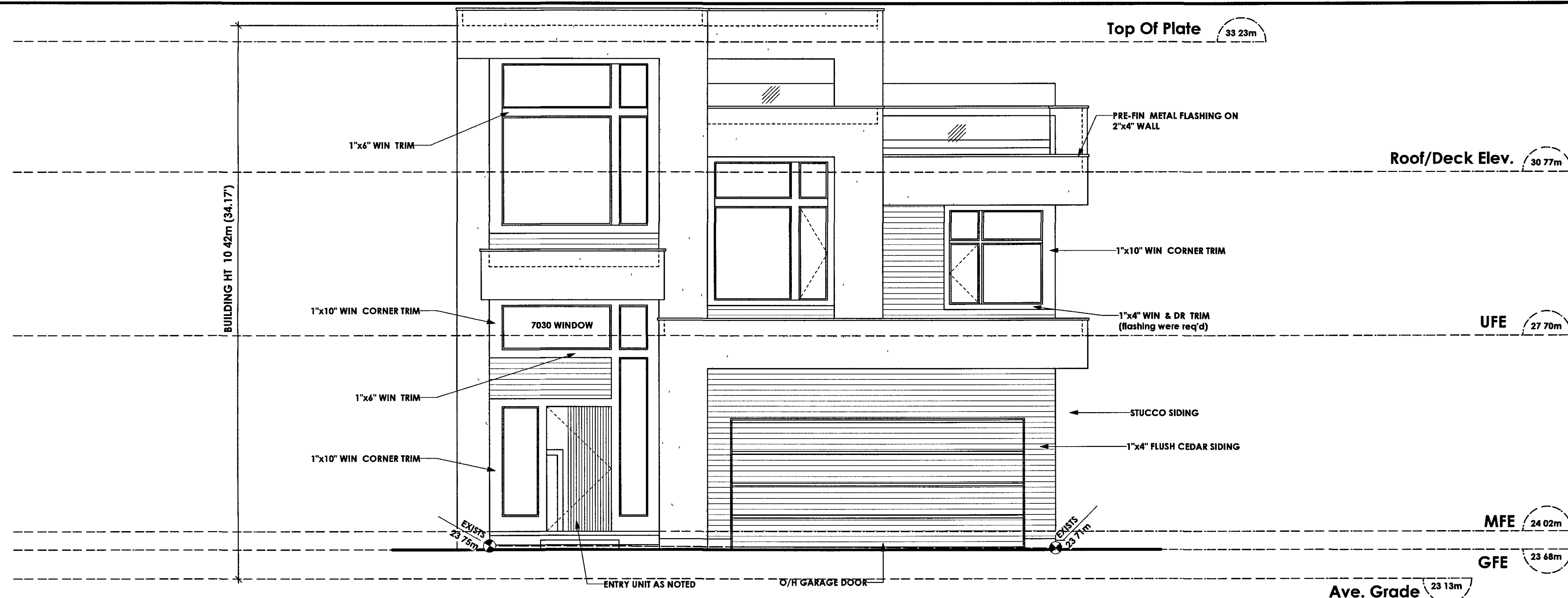
1 Front Elevation A2 Scale: 1/4" = 1'-0" AVE GRADE: ((23.43 + 23.43) ÷ 2) X 10.67 = (47.46) X 10.67 = 253.199
