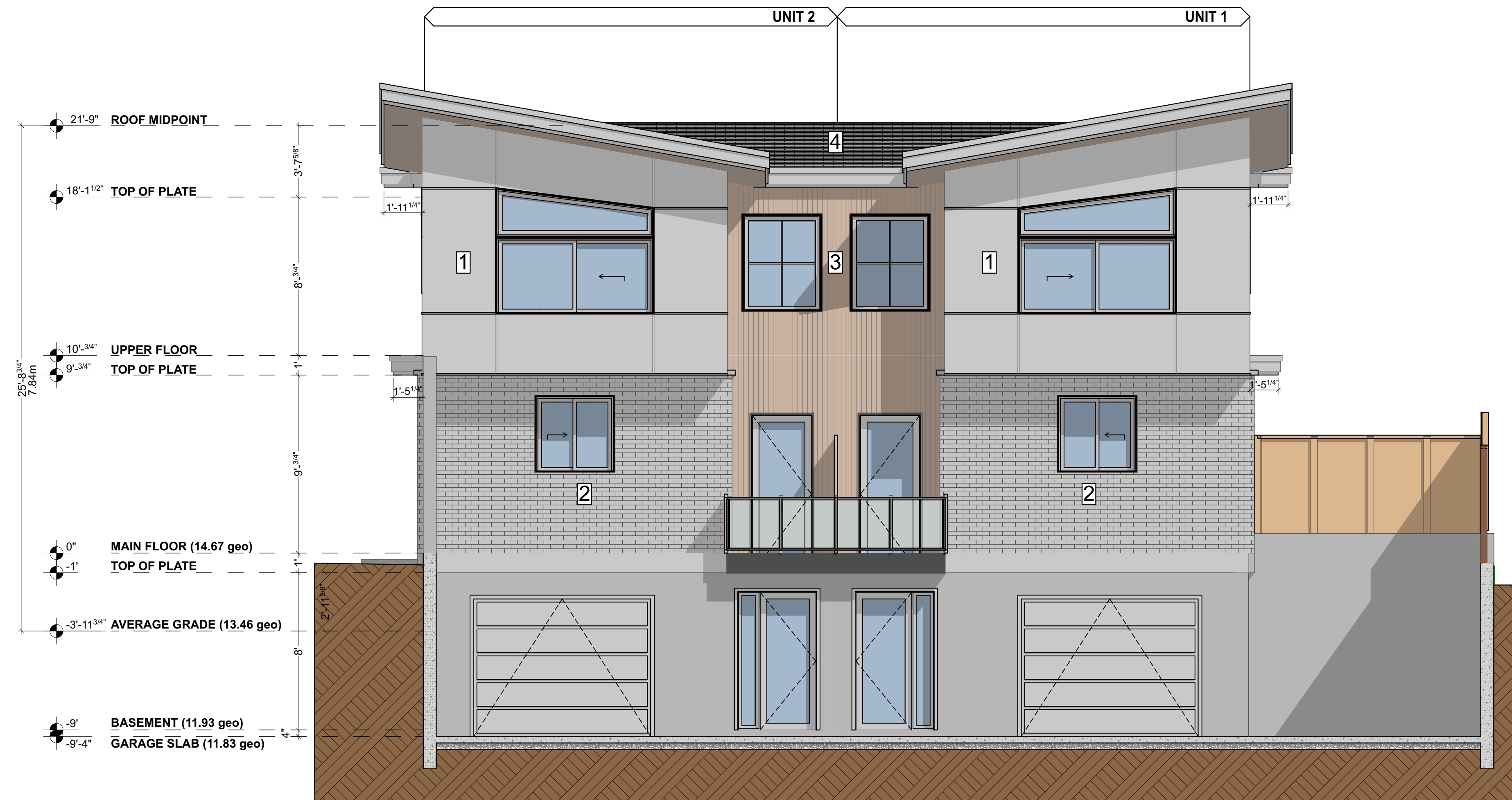
1 NORTH ELEVATION BLOCK B SCALE: 1/4" = 1'-0"
