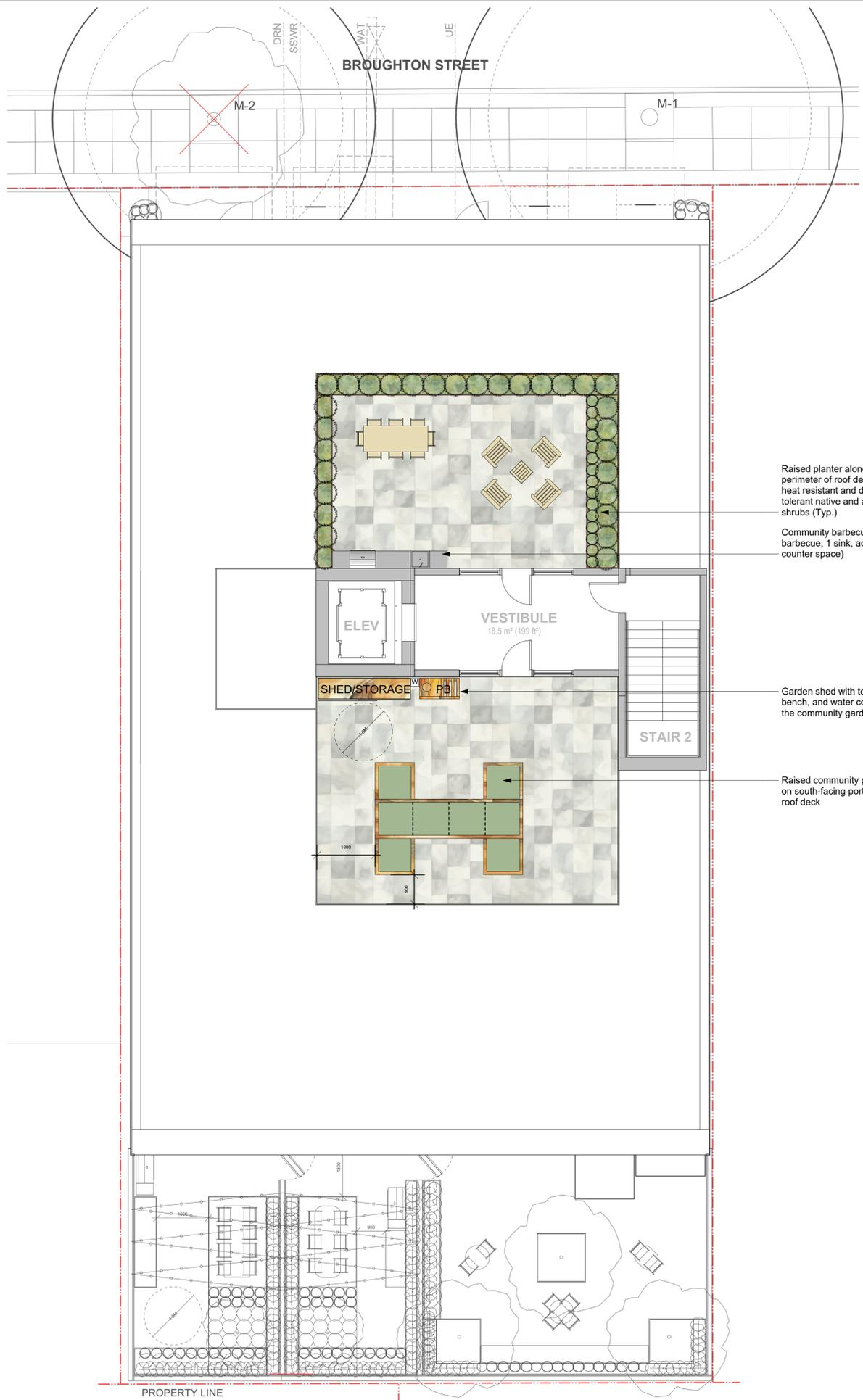
Raised planter along perimeter of roof deck with heat resistant and drought tolerant native and adaptive shrubs (Typ.)
