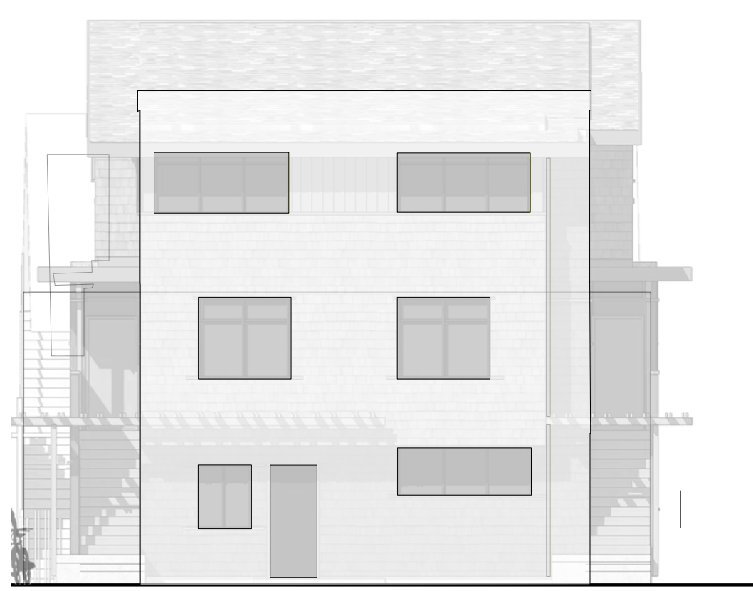
Face A = 76.74m 2 Unprotected Openings = 15.95m 2
