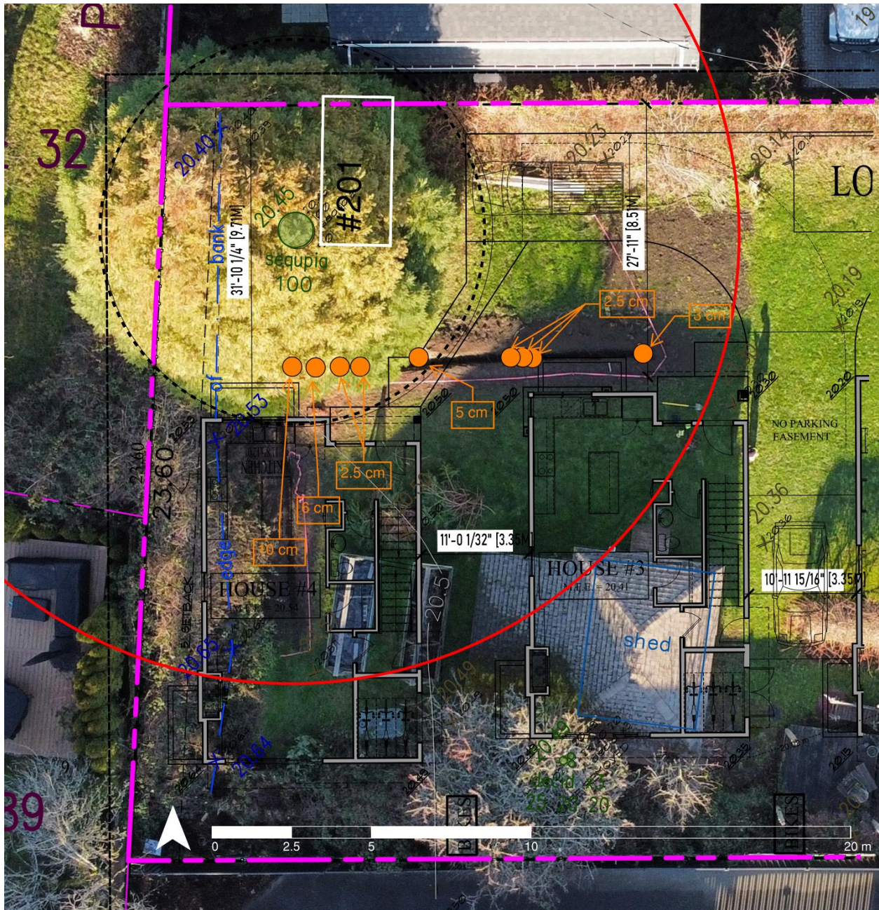
Figure 13. Aerial photo of exploratory excavation (obtained January 29, 2025), root locations, and root size.
