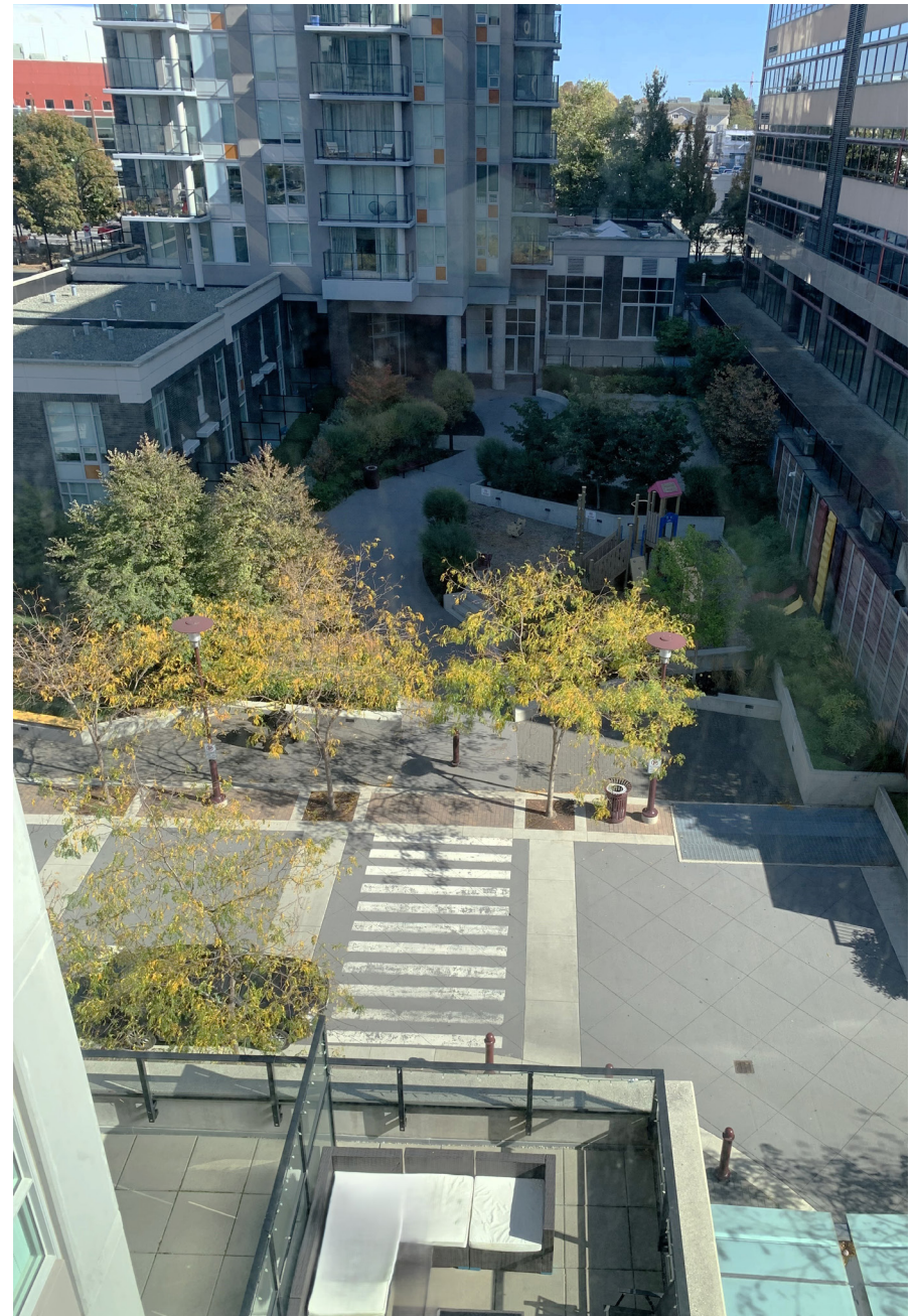
Short-term parking and loading areas are differentiated from pedestrian areas by surface materials, trees and urban furniture at a mixed-use residential development.
