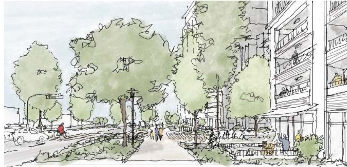
Conceptual illustration of the Loop along the Blanshard frontage. The pathway is physically separated from the roadway and runs between a double row of trees providing an interstitial frontage for the ground-oriented residential units. Modifications to the street right-of-ways are ongoing in coordination with the City of Victoria.
