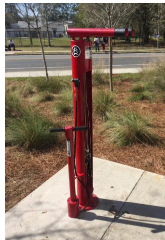
Example of an all-in-one bicycle maintenance station. (Image source: Dero, Kearney Centre)
