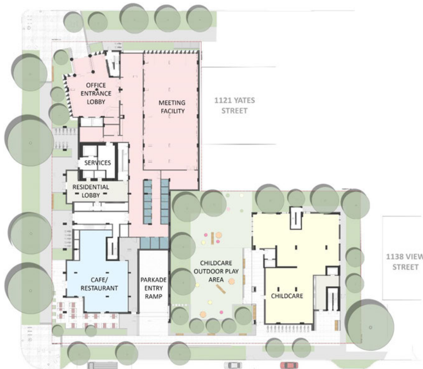
Site Plan: Yates Street is the address and front door to the meeting facility and upper floor offices. The West Residential entrance is located mid-block on Cook Street, and at the corner of Cook and View Streets is a café with patio. Along View Street, there will be the entrance to underground parking and services, the childcare outdoor play area and entrances to the East building (licensed child care and the residential lobby).
