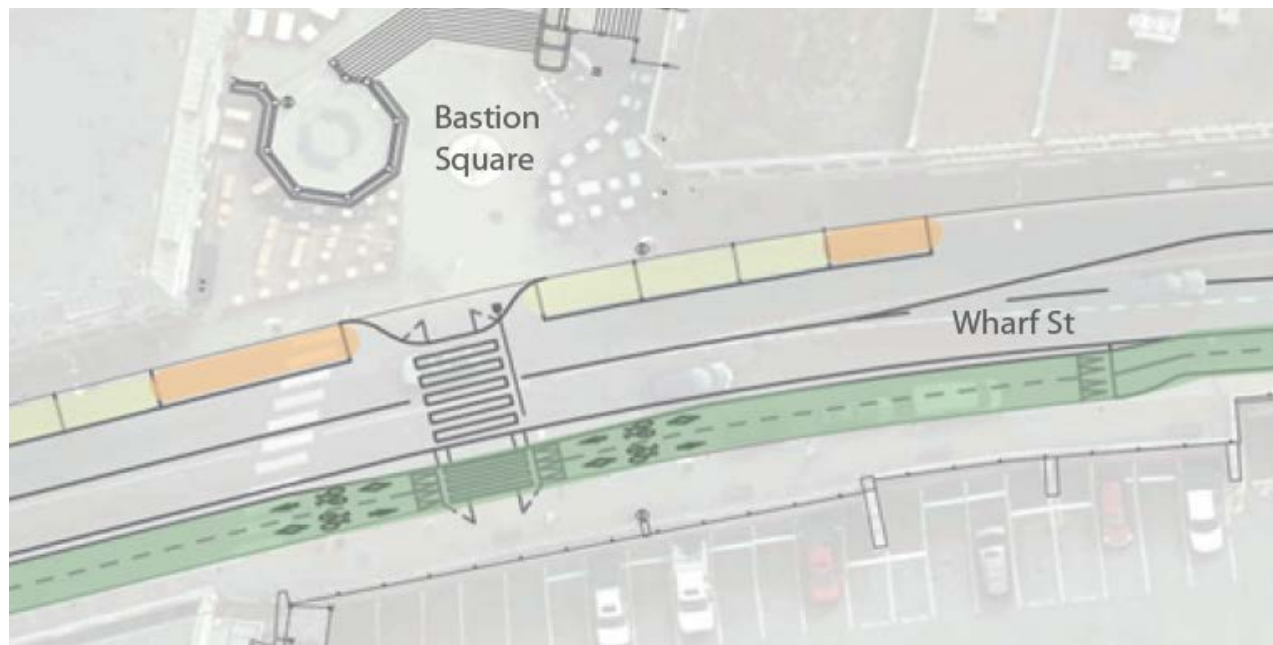
Figure 5: Bastion Square pedestrian crossing and replacement of on-street parking on 1200 block with bike lane
