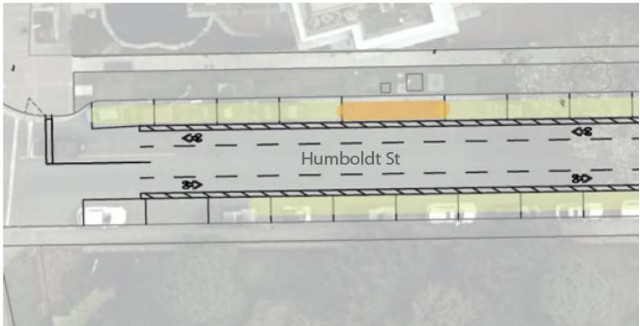
Figure 16: Advisory bike lanes - the treatment, applied to the full length of the block, is intended to help motorists and cyclists safely position themselves in the roadway.
