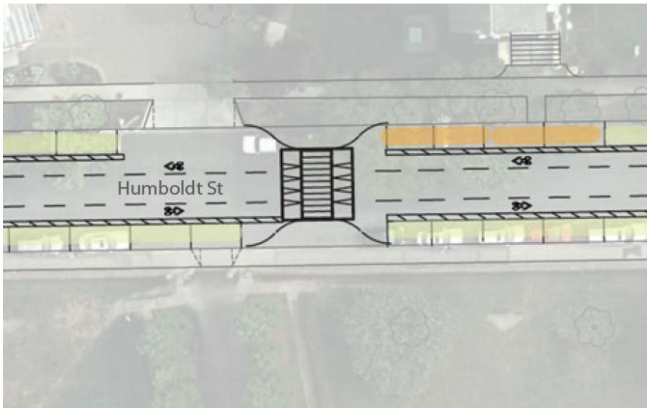
Figure 17: New raised pedestrian crossing to improve safety and visibility on the 800 block Humboldt Street
