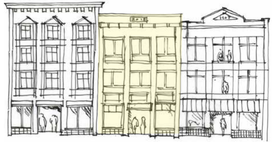
Illustrative example of a new infill building (in yellow), complementing the existing pattern, placement, spacing and proportions of windows, entries, structural bays and other architectural elements.
