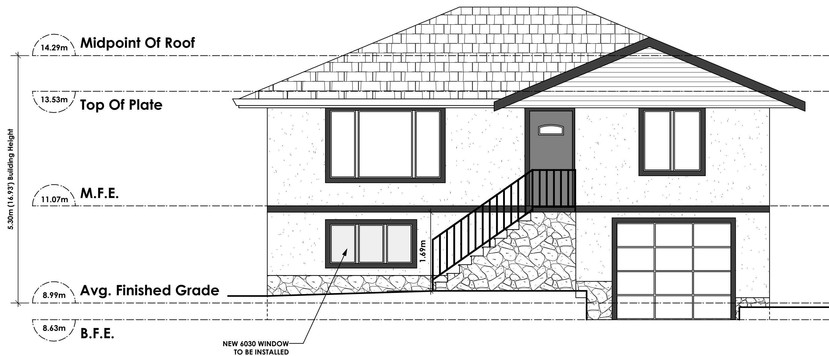
1 Front Elevation Scale: 1/4" = 1'-0"
