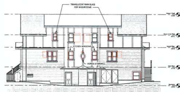
House A West Elevation with House B Windows Overlayed ⑥ 1:100
