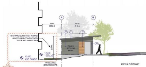
1 East Bike Storage West Elevation Scale: 1/100
