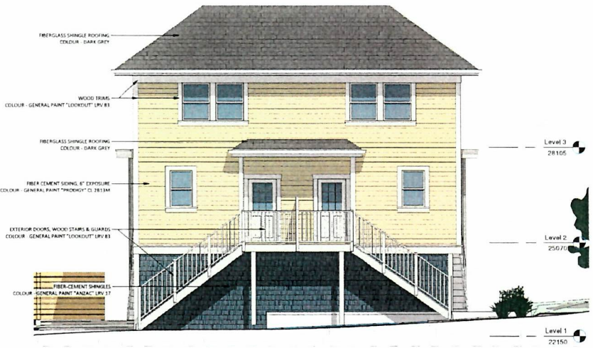
2 West Elevation - Building A 1:50
