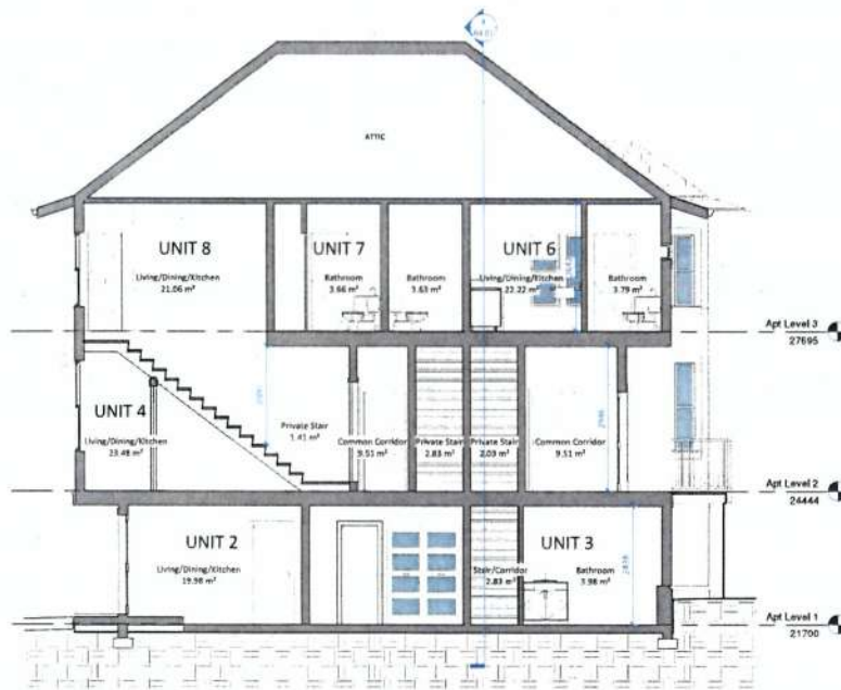
3 Building B Section A-A 1:50
