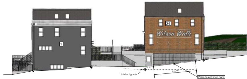
A14 3 EAST ELEVATION (FROM ALSTON) scale: 1/8" = 1'-0"
