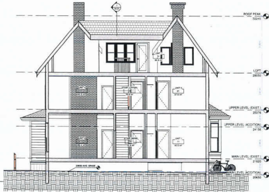
2. BUILDING SECTION - E-W (FACING S) @ EXISTING HOUSE 1:50
