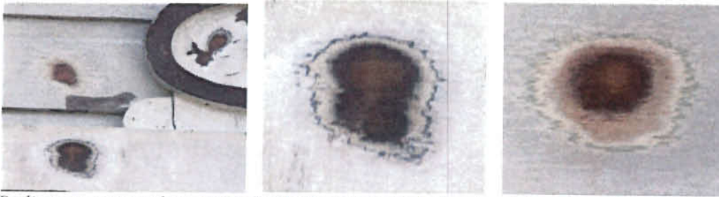
Preliminary paint colour testing by 'bulls-eye' method, showing different paint layers. This investigation was followed by extensive paint sampling for microscopic analysis.
