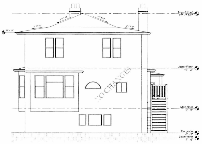
Existing Front Elevation 1/4" = 1'-0"
