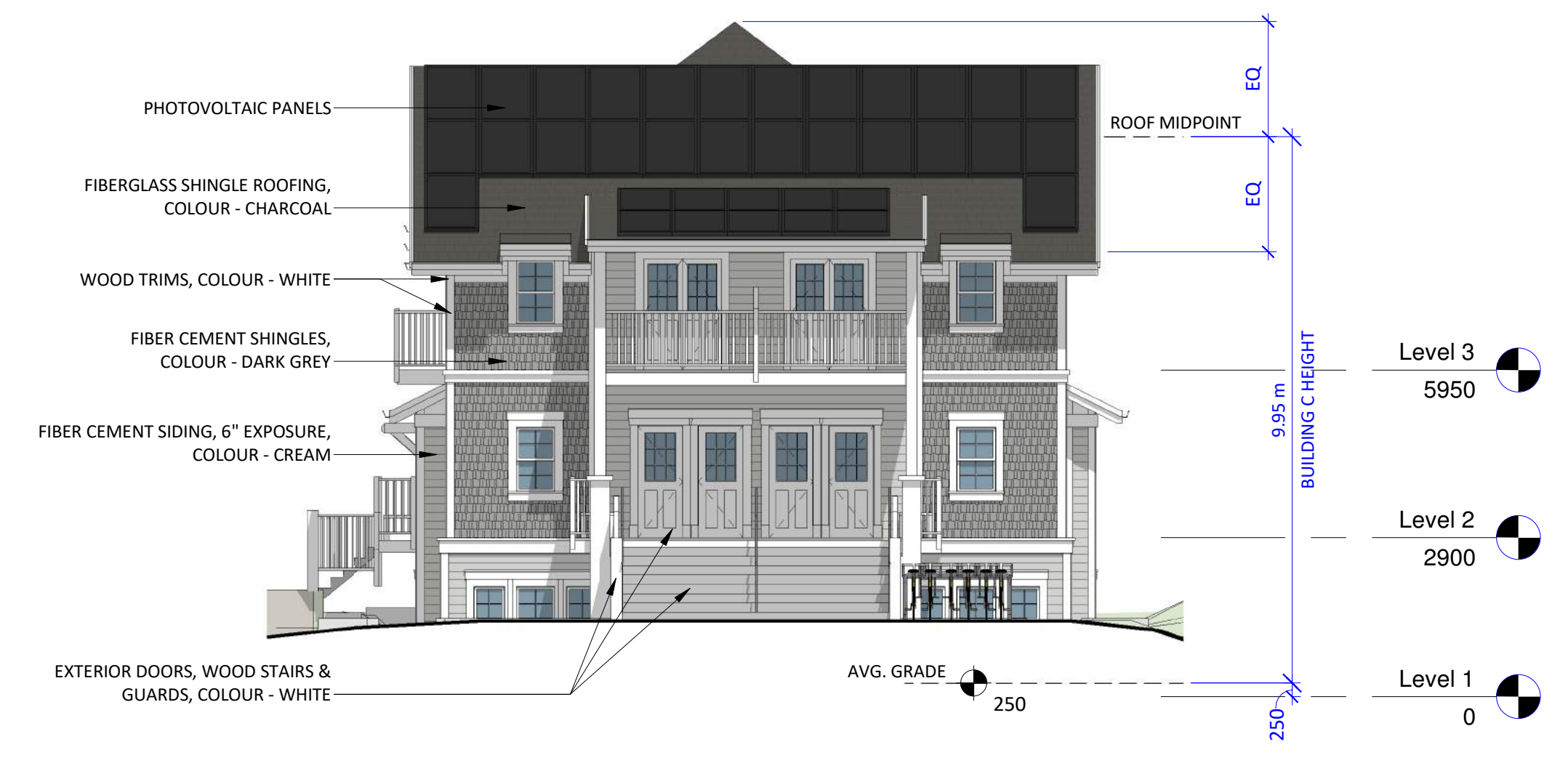
2 South Elevation - Building C 1 : 100
