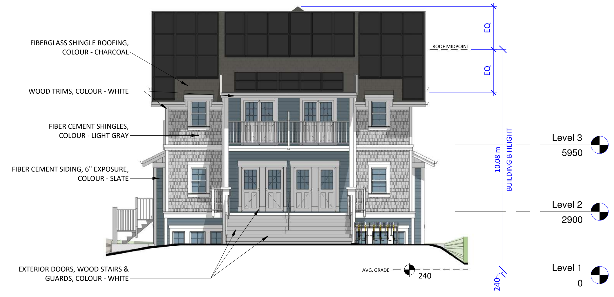
3 South Elevation - Building B 1 : 100
