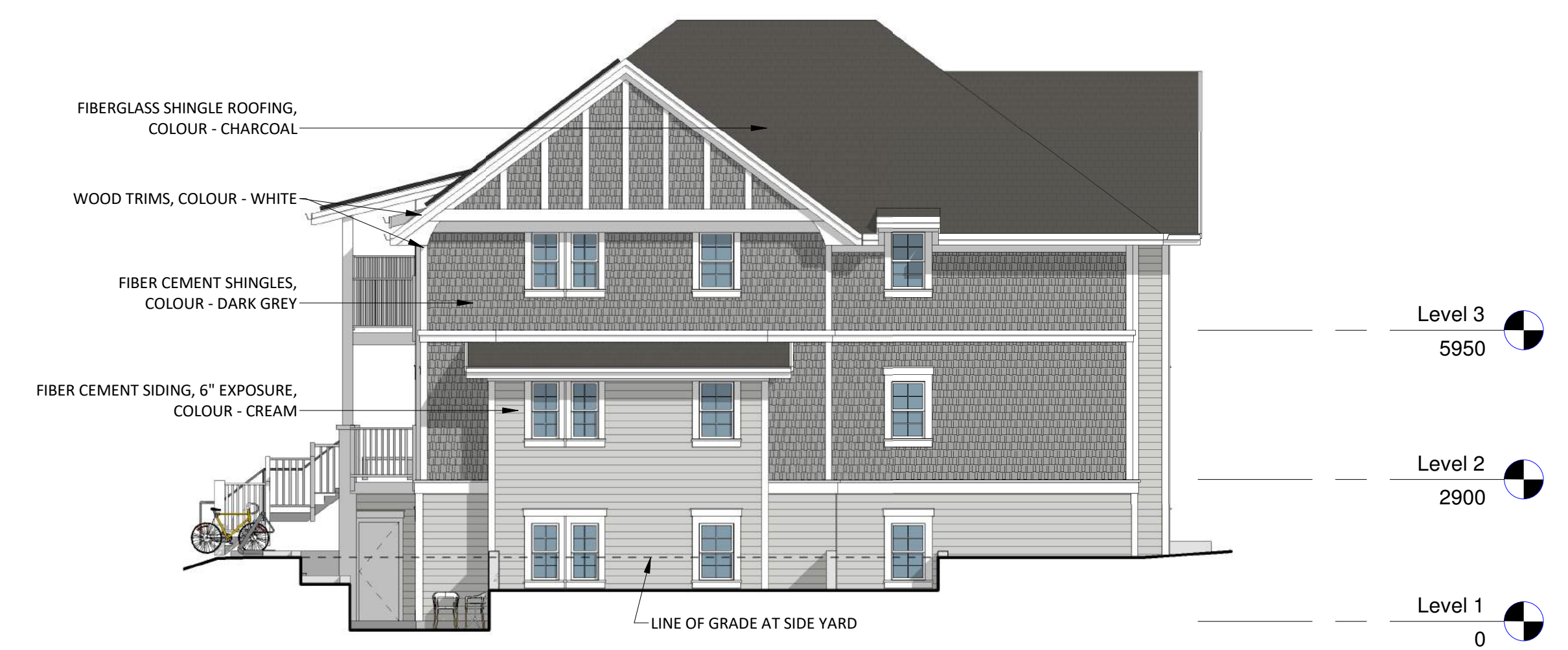
3 East Elevation - Building C 1 : 100
