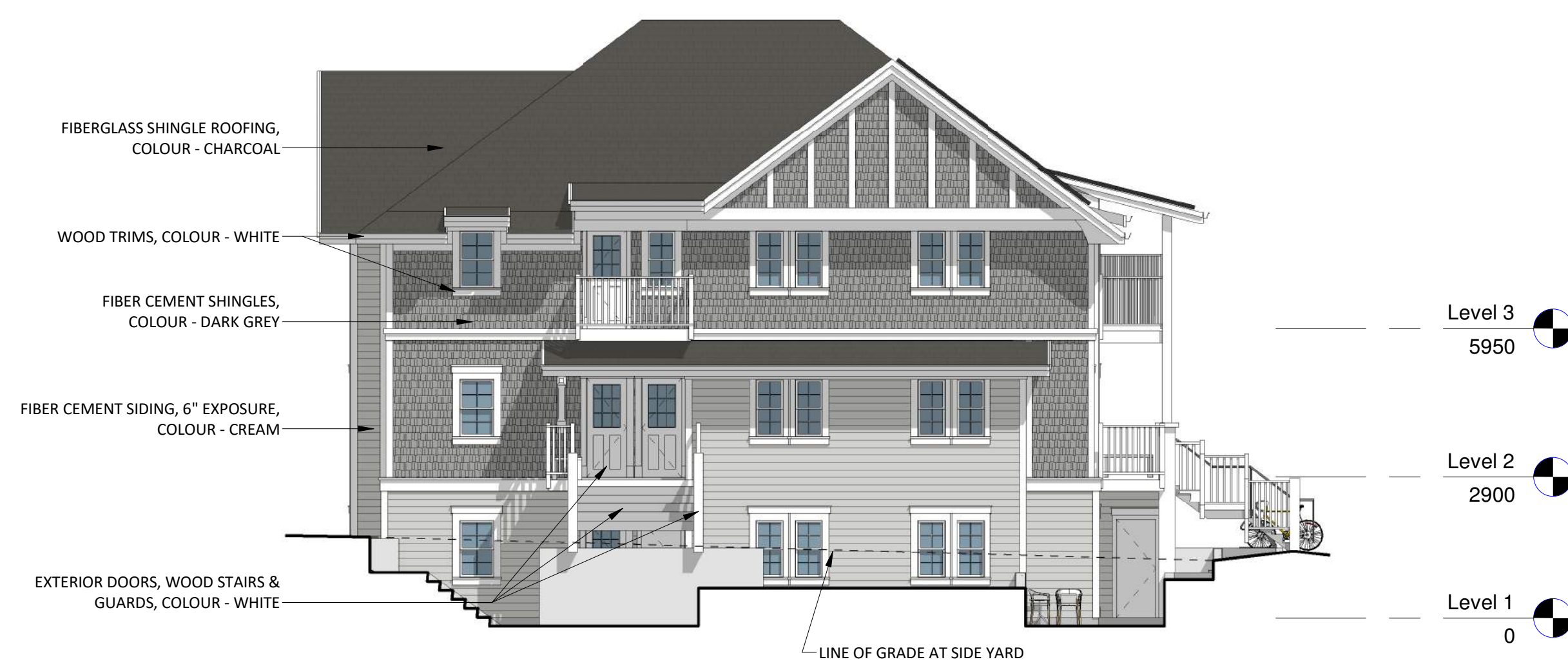
4 West Elevation - Building C 1 : 100
