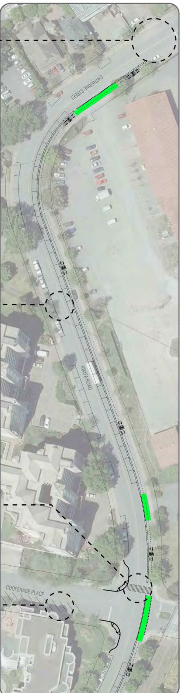
Kimta Road | Catherine Street to Saghalie Road - preliminary design concept for advisory bike lanes
