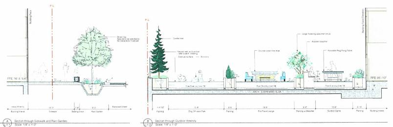
Section through Sidewalk and Rain Garden Scale 1/4" = 1'-0"
