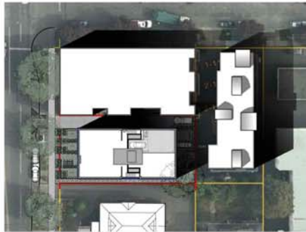
3 Site Plan Shadow Study A1.3 June 21st at 3PM 73° from S, Azimuth 46.5° from horizon not to scale
