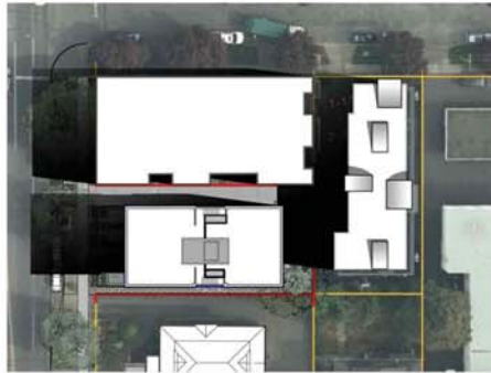
1 Site Plan Shadow Study A1.3 June 21st at 9AM 73° from South, Azimuth 46.5° from horizon not to scale
