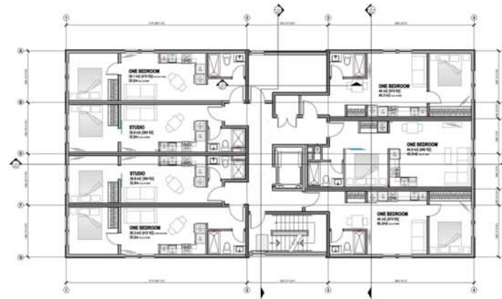
3 2nd, 3rd, 4th, and 5th Floor Plans metric scale 1:100
