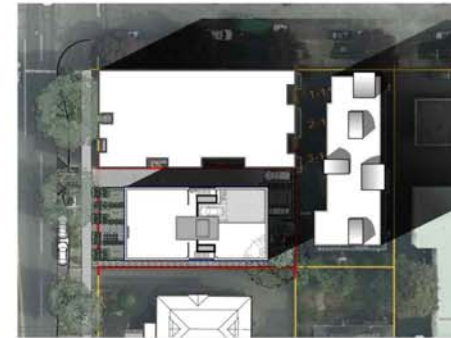
6 Site Plan Shadow Study A1.3 March 21st and September 21st at 3PM 54° from S, Azimuth 27.5° from horizon not to scale
