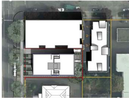
2 Site Plan Shadow Study A1.3 June 21st at 12 Noon 0° from S, Azimuth 65° from horizon not to scale
