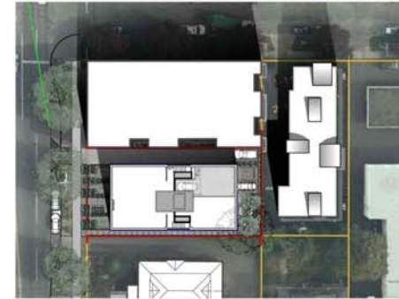
5 Site Plan Shadow Study A1.3 March 21st and September 21st at 12 Noon 0° from S, Azimuth 41.5° from horizon not to scale
