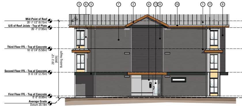
② South Elevation - Building A Scale: 1:100
