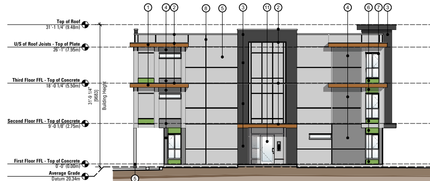
② South Elevation - Building B Scale: 1:100
