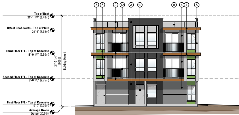
③ West Elevation - Building B Scale: 1:100
