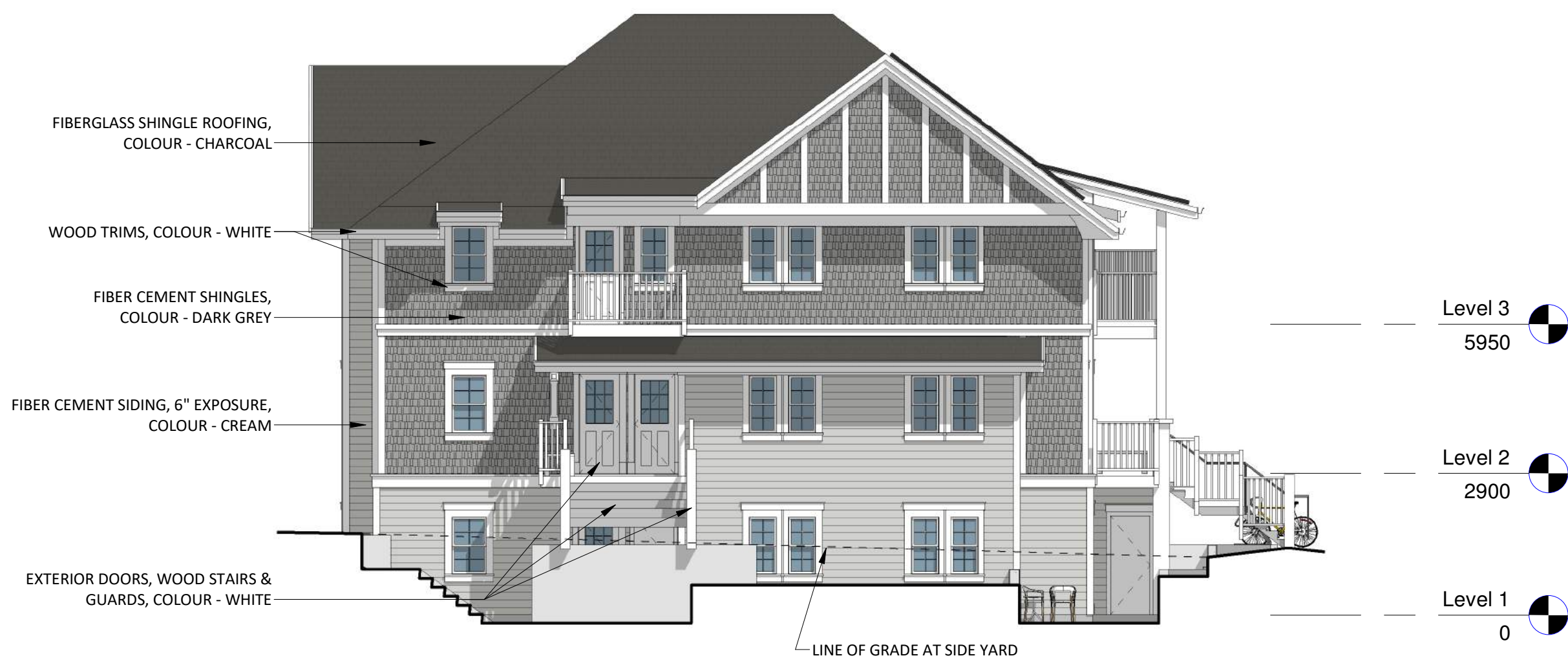
4 West Elevation - Building C 1 : 100
