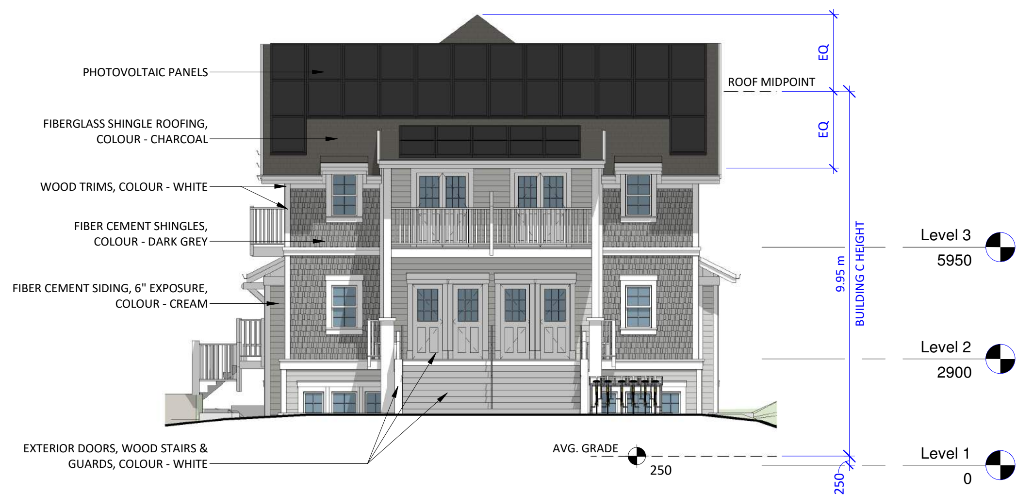
2 South Elevation - Building C 1 : 100
