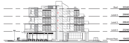
① East Elevation - Limiting Distance SCALE = 1 : 300
