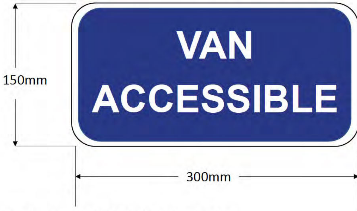
Figure 2: Recommended Blue and White “Van Accessible” tab
