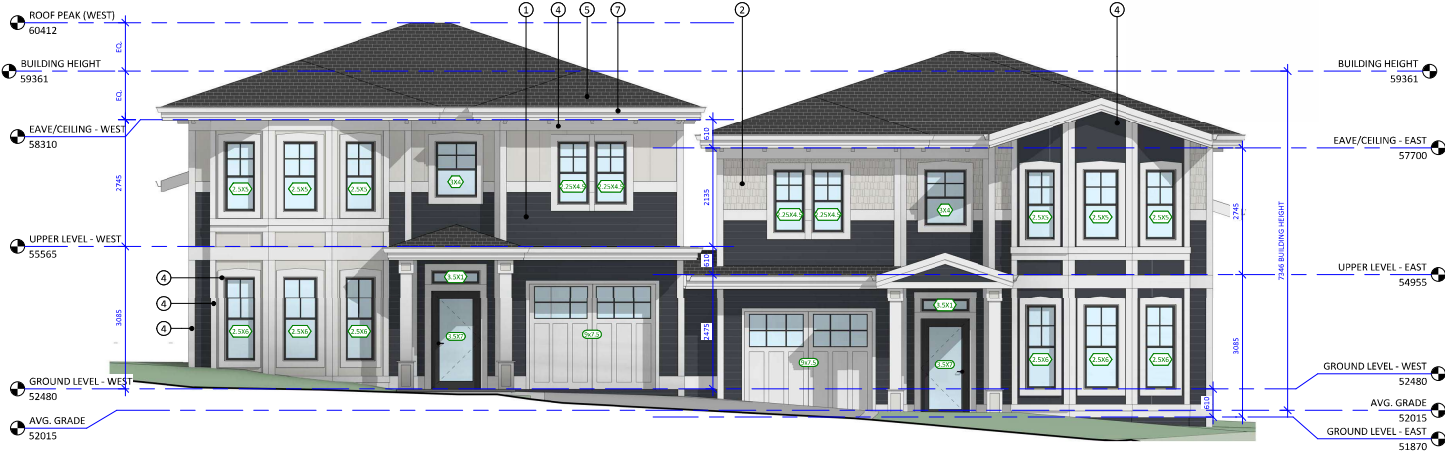
1 BUILDING ELEVATION - SOUTH 1:50
