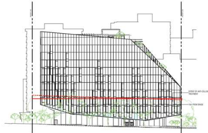
Elevations showing the extent of anti-collision treatment
