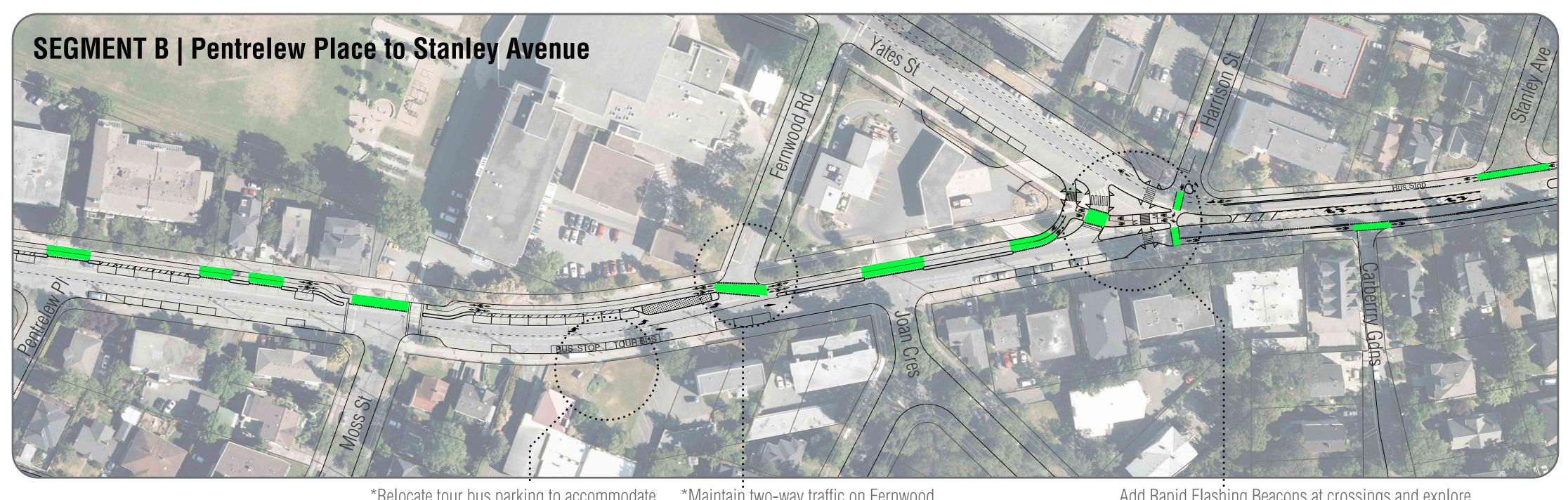
\*Relocate tour bus parking to accommodate fire truck turning movements
