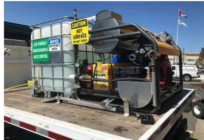
Heated Organic weed treatment unit designed & built by Public Works
