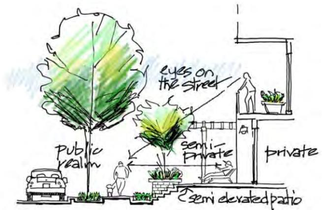
Diagram showing incorporation of entries to individual ground floor units that are clearly visible from the fronting street.
