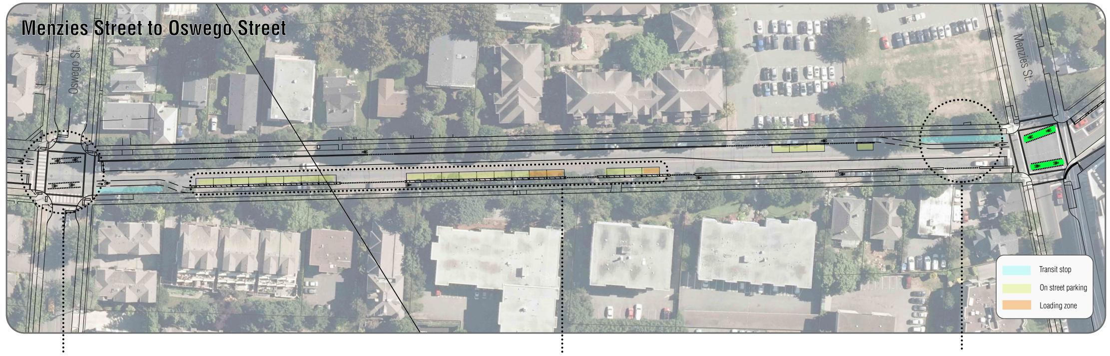
Add paint markings for pedestrians and cyclists and improve crossing with new curb bulb outs and let downs One-way protected bike lanes with parking retained on the southside of the street
