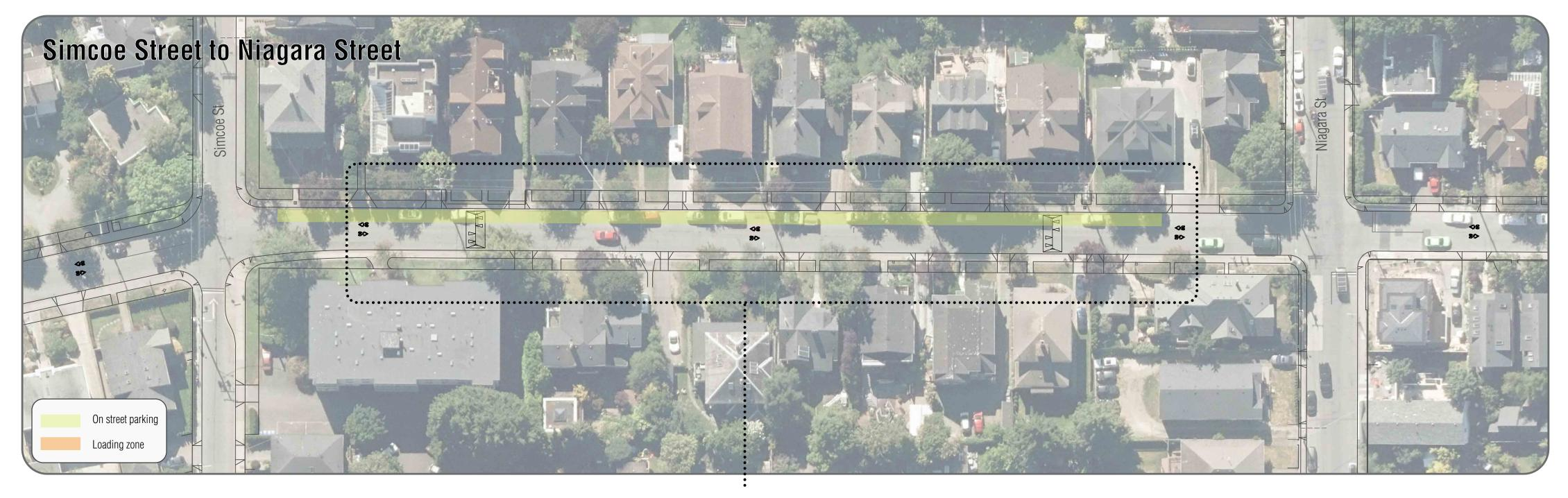
Add speed humps, 30 km/hr speed limit and sharrow paint markings
