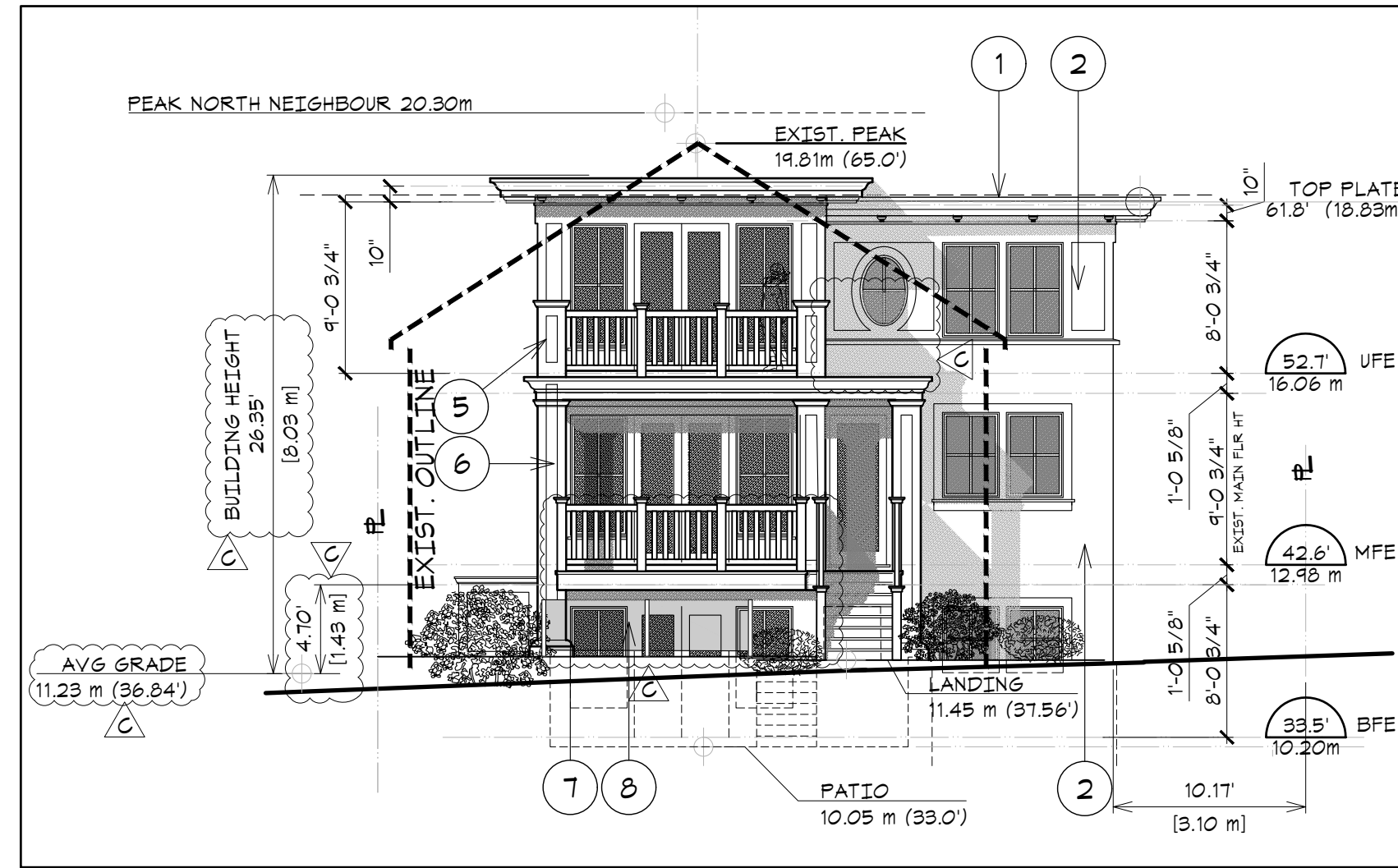
1 EAST ELEVATION SK-2 SCALE: 1:100 HOLLYWOOD CRESCENT
