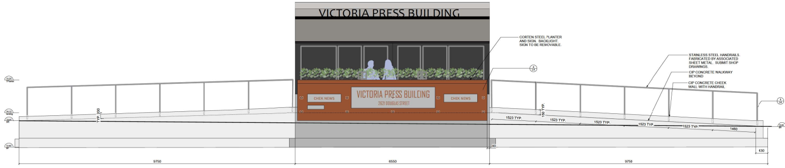
2 Elevation - Front Landing/ Ramp/ Handrails Scale: 1:30
