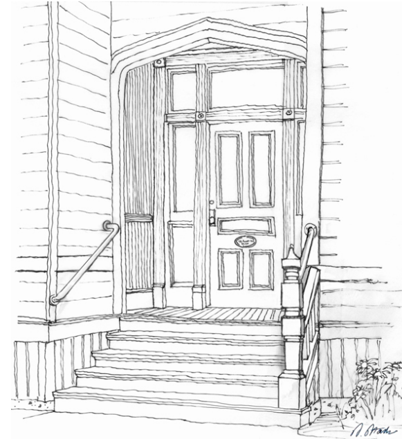
Heritage Consultant Stuart Stark's design for a code compliant railing on 1139 Burdett Street. The design uses a simple pipe rail extending from the house to the newel post
