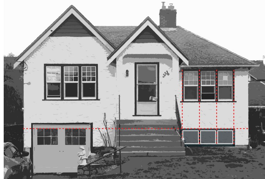
Align new basement windows with upper storey windows and include the same number of vertical divisions.
