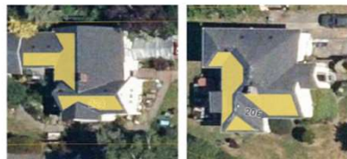
Possible areas for rooftop solar arrays
