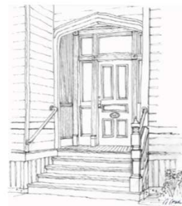
Heritage Consultant Stuart Stark's design for a code compliant railing on 1139 Burdett Street. The design uses a simple pipe rail extending from the house to the newel post
