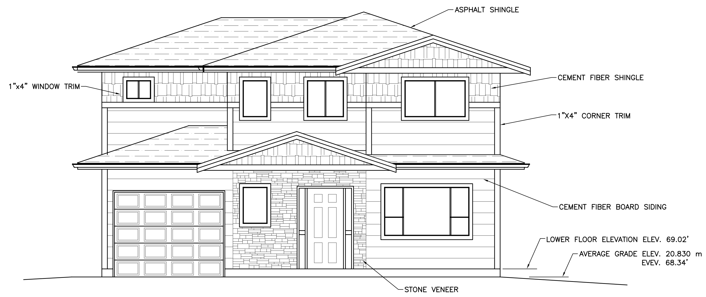
EAST ELEVATION – LOOKING WEST SCALE: 1/4" = 1'-0"
