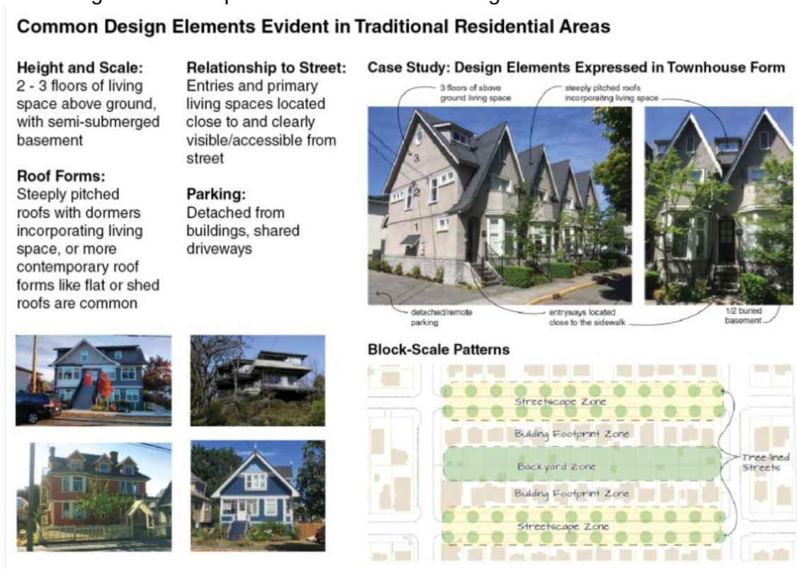
Figure 5 - Key pattern and design elements common to Traditional Residential areas that help buildings relate positively to the street, support livability, social interaction, and neighbourliness.
